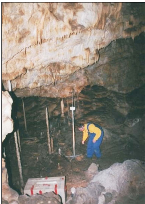
Photo 3. Acoustic anemometer at measurement point in the Bamboo Grove area. Photo: J. Piasecki
