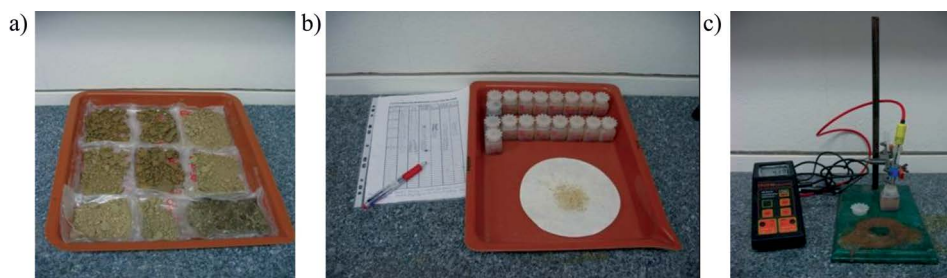
Fig. 2. Works in laboratory: a) drying of soil samples; b) preparing of soil leachates; c) pH measuring
