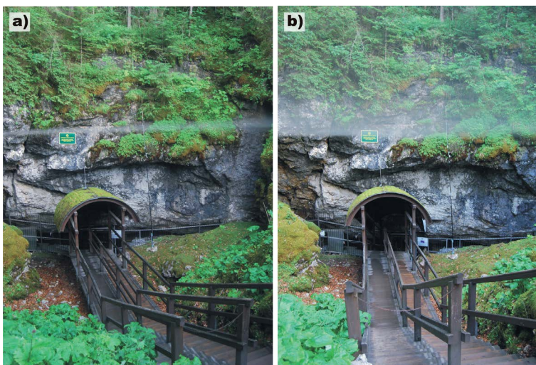
Fig. 16. Condensation layer formed above the Entrance Collapse of Dobšinská Ice Cave: a) situation before start of the ‘open door’ experiment; b) the state of condensation layer after two hours of experiment. Photo: T. Sawiński, July 2012
